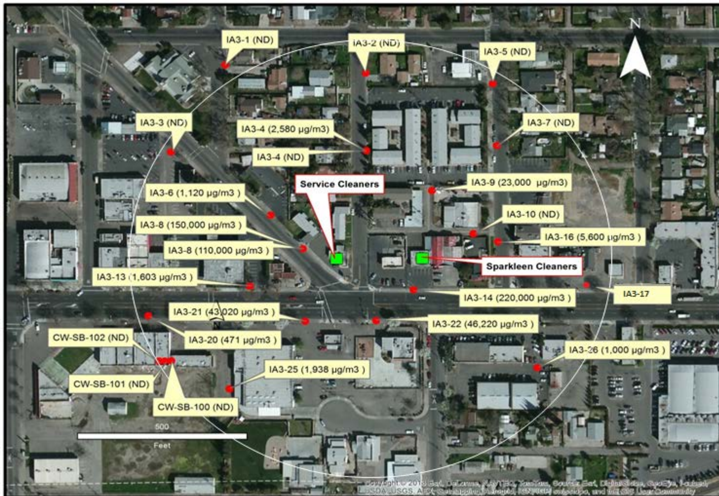
Figure A3: PCE Concentrations in soil gas at 5 feet depth within a 500 feet radius of Service and Sparkleen (2001-2003)
