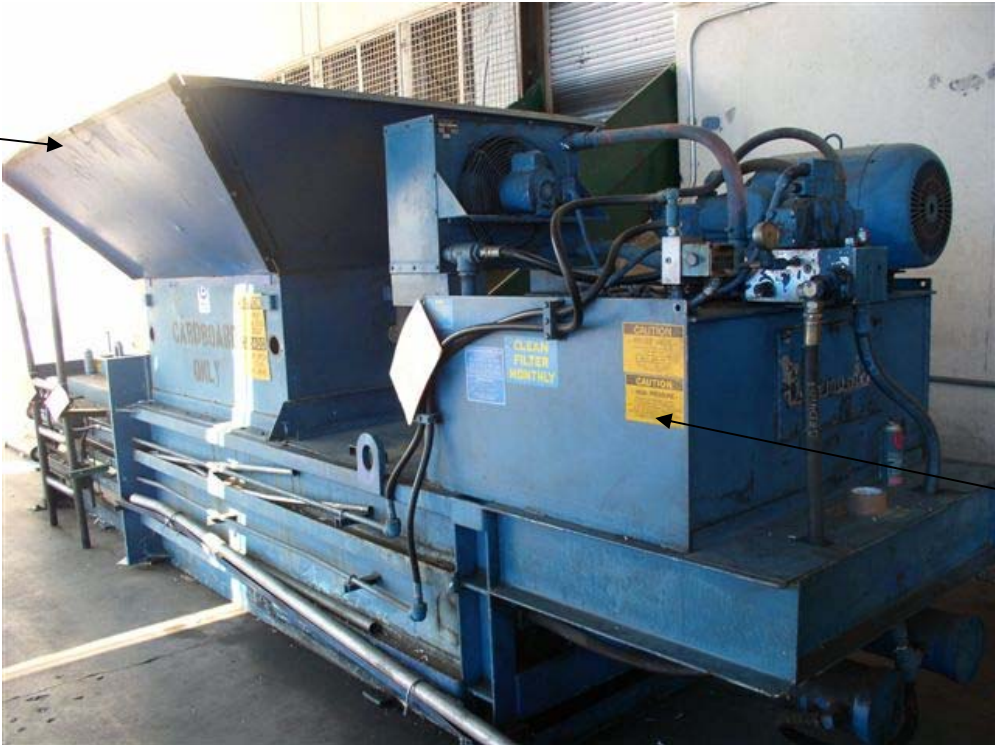
Exhibit 2. The cardboard baler showing the hydraulic system and feed chute.
