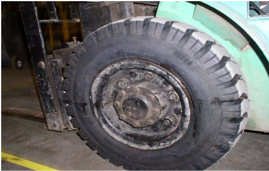
Exhibit 1. A forklift multi-piece rim and tire assembly similar to the one involved in the incident.
