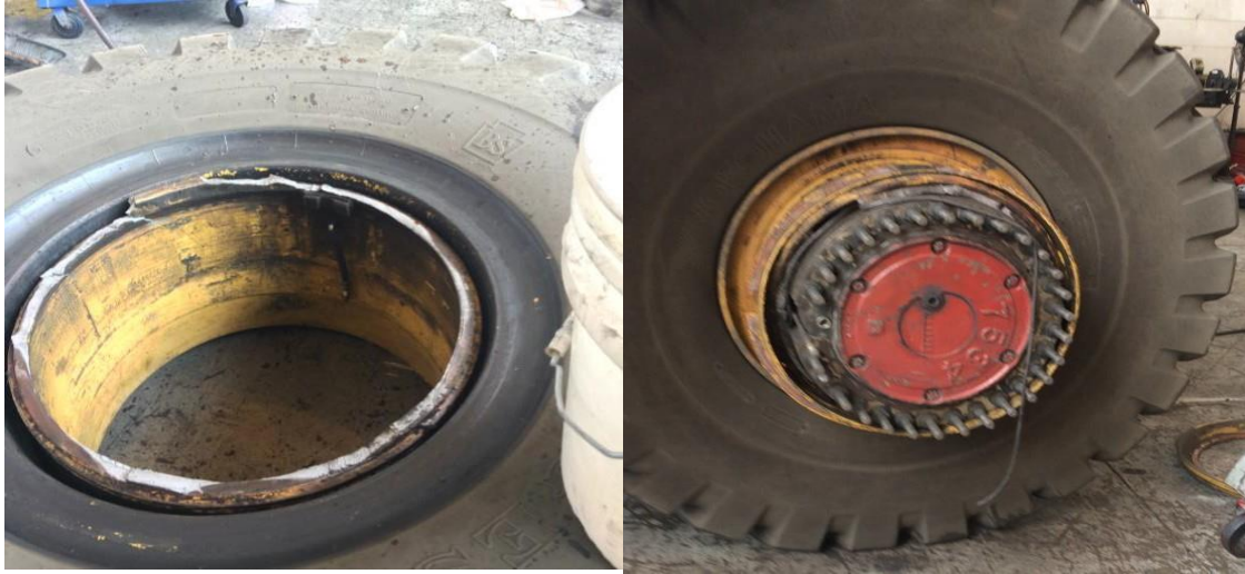
Exhibit 7 & 8. The outer (left) and inner (right) tires on the container handler after the incident.
