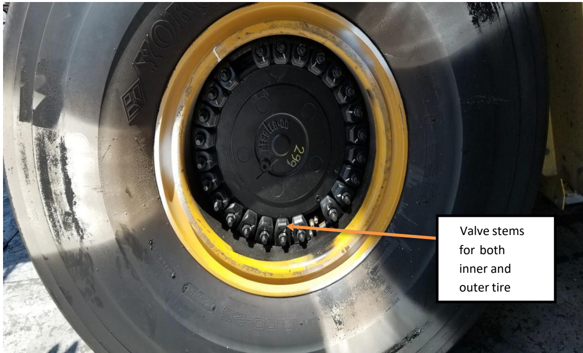
Exhibit 3. A tire and wheel assembly similar to the one involved in the incident, including valve stems and 24-bolt pattern holding the wheel assembly together.
