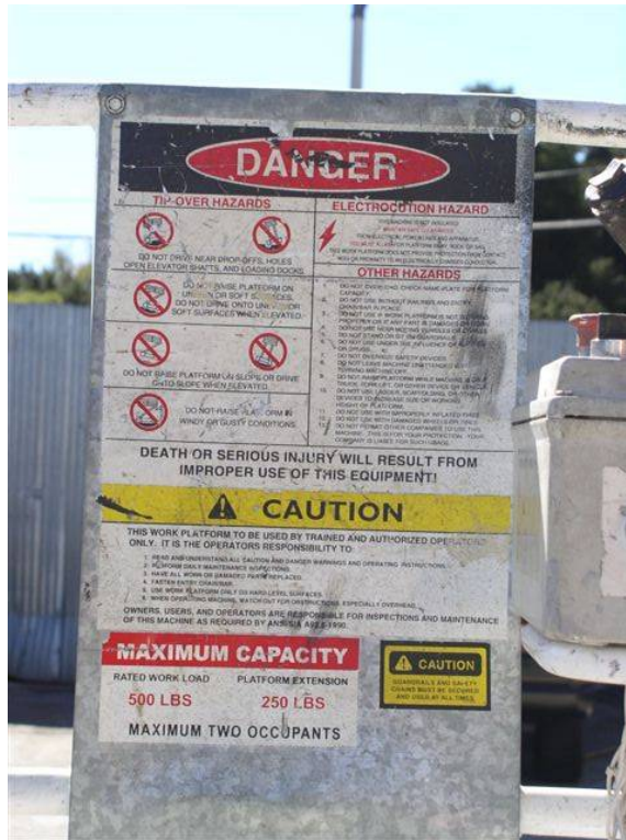
Exhibit 3. The placard attached to the scissor lift listing hazards associated with operation.
