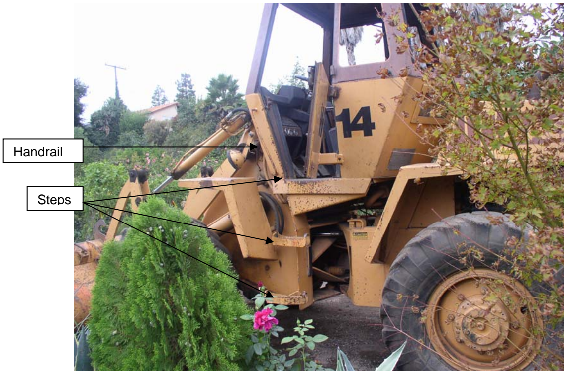
Exhibit 2. The stairs and handrail used to gain access to the cab.
