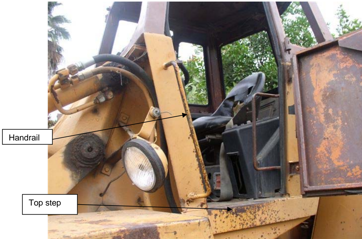
Exhibit 3. The entrance to the cab of the tractor showing the top step and handrail.
