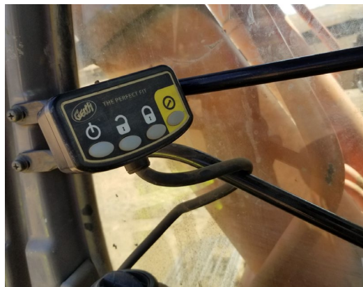
Exhibit 3. The automatic hydraulic quick coupler control panel.
