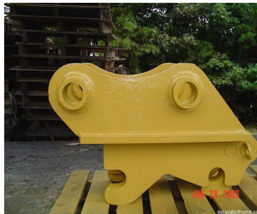
Exhibit 2. A quick coupler similar to the one involved in this incident.
