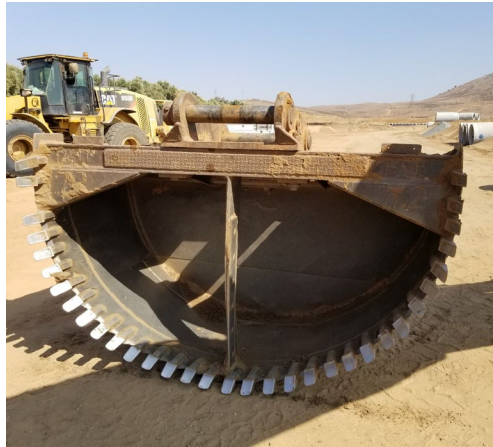
Exhibit 4. The bucket that disconnected from the coupling.
