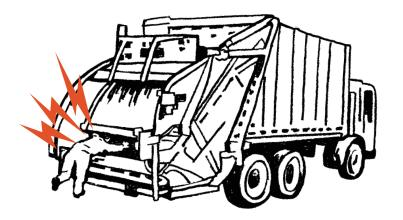
In recent incidents, two laborers, Marcos B.\* and Pete S.\*, died while collecting trash. Both were crushed by hydraulic equipment on trash trucks. In both cases, co-workers started the equipment before checking to see if anyone could be struck by the moving equipment. Marcos was crushed by hydraulic arms when they were lowered to the front of a truck to pick up a container. Pete was crushed by the compactor panel of a truck when it started to compact some trash.
